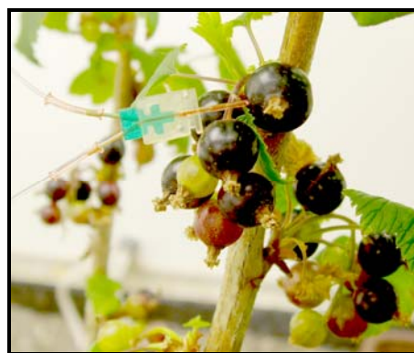
Figure M6 A diagrammatic illustration of the micro-dialysis (MAB 6) probe Microbiotech, Sweden (left) and an image of a probe mounted in an attached berry with perfusion solution being supplied to the fruit via the upper tube and the resultant exudate from the from being collected via the lower tube (right)
